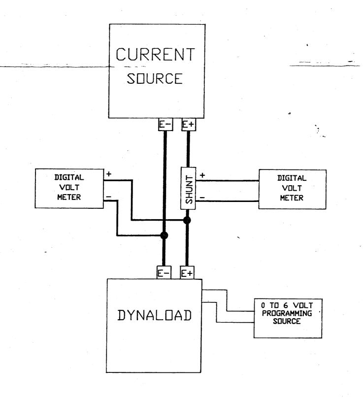
FIGURE 1. CALIBRATION SETUP
